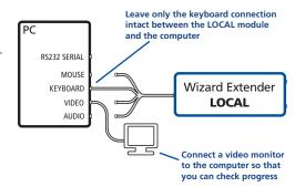
4 So that you can check upgrade progress, connect a monitor directly to the video port of the computer.
